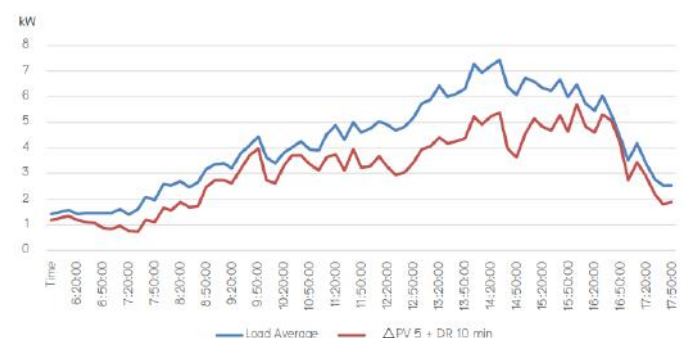
Fig. 7 : The use of DR program in 10 minutes use with the electricity generating set from 5 kWp solar photovoltaic cell
